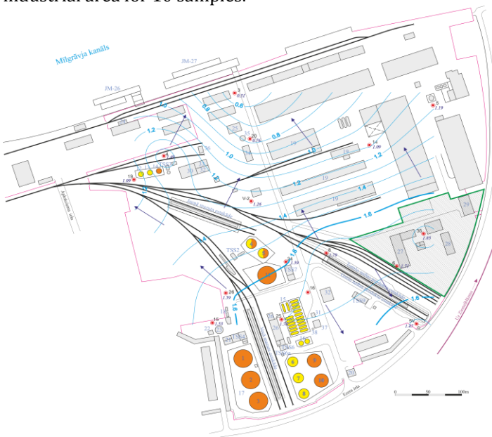
Fig. 1. Study and pilot research area (marked with green). Groundwater flow directions are shown as arrows.
