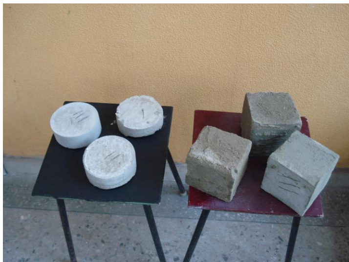
Fig. 2. Solidified soil samples for compressive strength and freeze thaw resistance studies.
